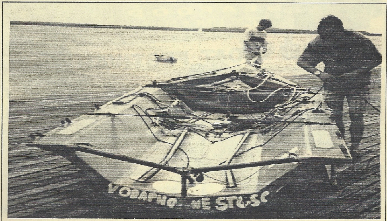
Modern 16' skiffs are of high tech carbon fiber. This is just the hull before rigging at Botany Bay
