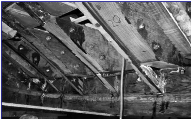
Above: The planks were tight-seamed with epoxy encapsulation, bonded to the frames and mechanically screwed with #16 silicon bronze wood screws.
