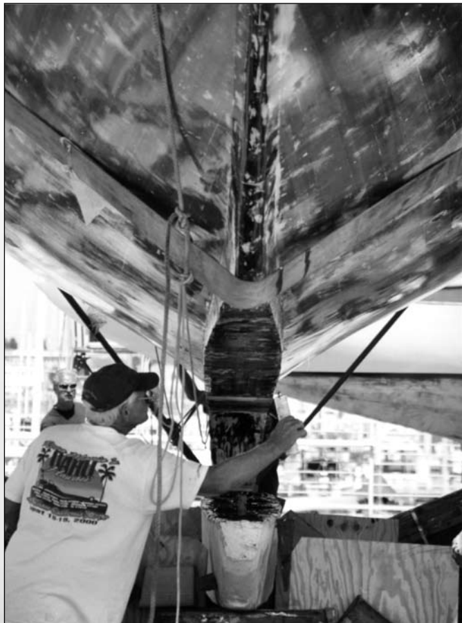
Right: Re-attaching the boat to the ballast keel required careful alignment with the crane, while the hull hovered over the keel on the cradle in the yard.
