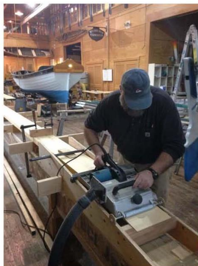
Orient mast under construction at the Port Townsend Wooden Boat Center.
