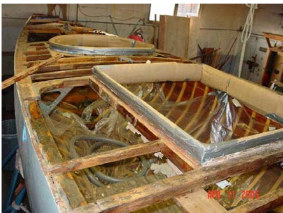
A new deck coming...
